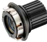
Shimano MS 612 POE Freehub Body STEEL + AL7075 6 springs & 6pawls 612 POE form Micro Shimano
